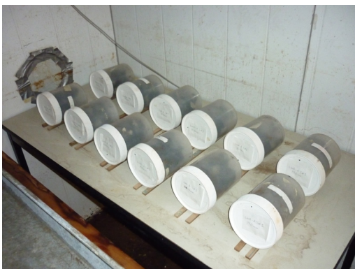
LWA samples undergoing freeze-thaw resistance testing
